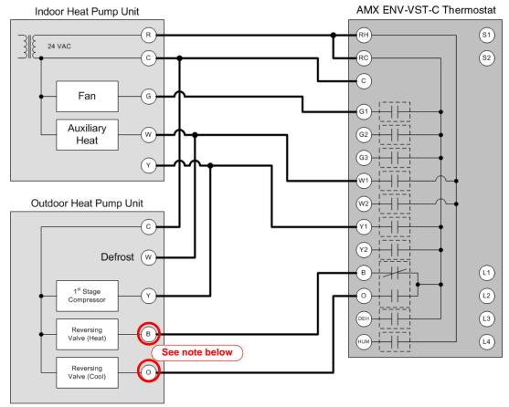
FIG. 8 Single Stage Heat Pump wiring
